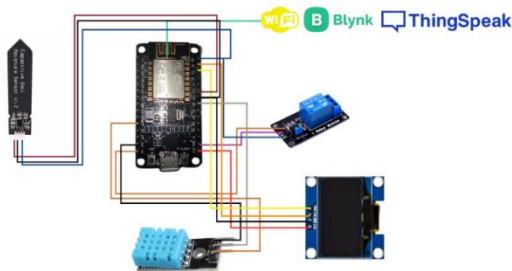
Gambar 10. Rangkaian Diagram Monitoring Sensor dan Kontrol Relay
