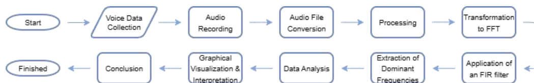
Figure 1. Research methodology flowchart for human voice frequency analysis using FFT and FIR
