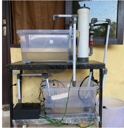
Figure 6. Implementation of the Laundry Wastewater Filtration Device
