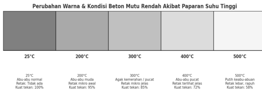
Figure 3. Illustration of color changes and surface condition of low-strength concrete after exposure to temperatures between 25°C and 500°C
