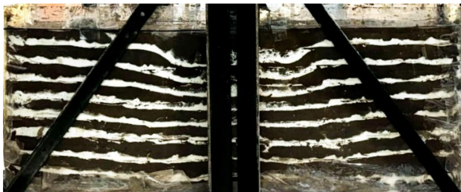
Figure 12. Failure pattern of cohesive soil under the finned slab sample with 90° inclination
