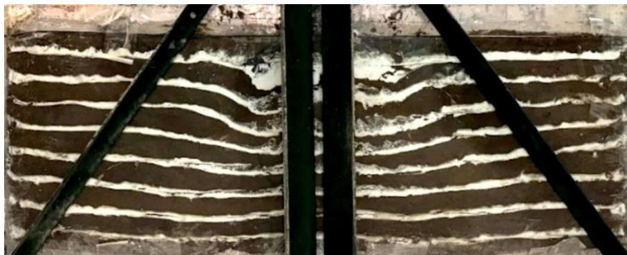
Figure 11. Failure pattern of cohesive soil under the finned slab sample with 60° inclination
