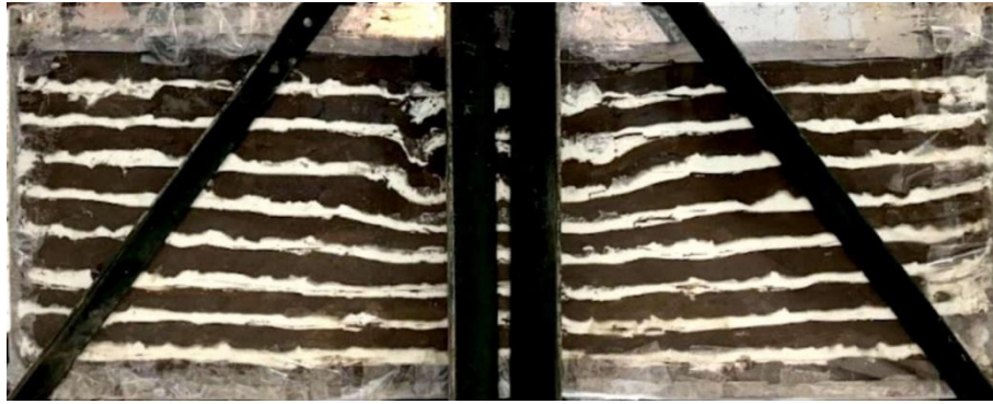
Figure 10. Failure pattern of cohesive soil under the finned slab sample with 30° inclination
