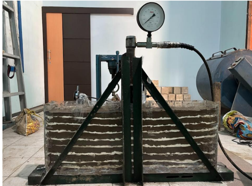
Figure 6. Front view of experimental tests of soil failure pattern
