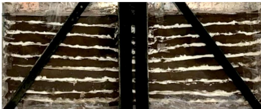
Figure 9. Failure pattern of cohesive soil under the finned slab sample with 0° inclination
