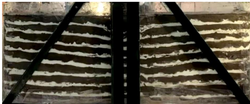
Figure 8. Failure pattern of cohesive soil under the unfinned slab sample
