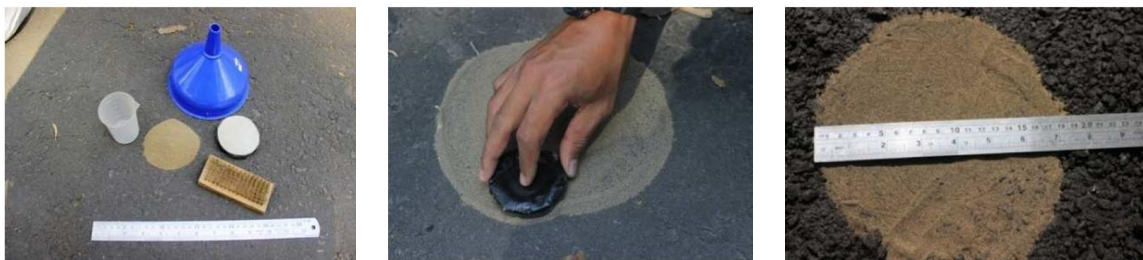
Figure 2. Texture Depth Testing with the Sand Patch Method [9]
