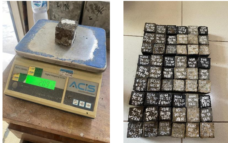
Figure 6 Bulk density sample
