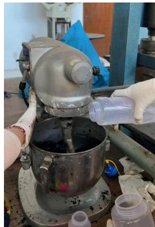
Figure 4 Mixing geopolymer binder
