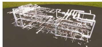
Figure 3. Mechanical Plumbing Model
