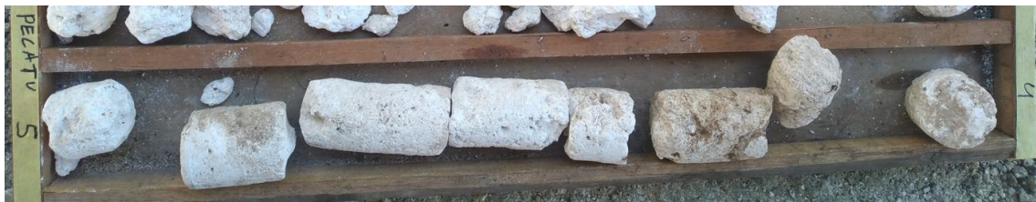
Figure 6. Core box of bore drilling result in Bingin Beach, Badung in 4-5 meter depth.
