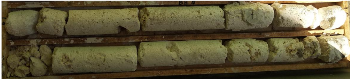
Figure 5. Core box of bore drilling result in Batu Meguwung Temple, Jimbaran, Badung.
