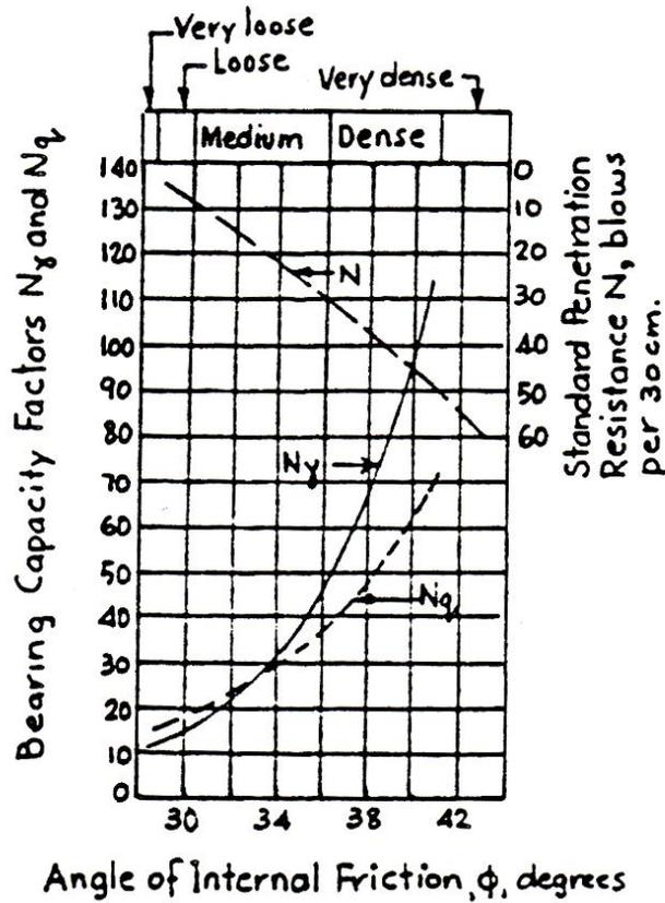
Figure 2. Graph of the relationship between bearing-capacity factors and  $\phi$ , and the empirical relationship of the standard penetration resistance value  $N$ . (After Peck et al (1974))
