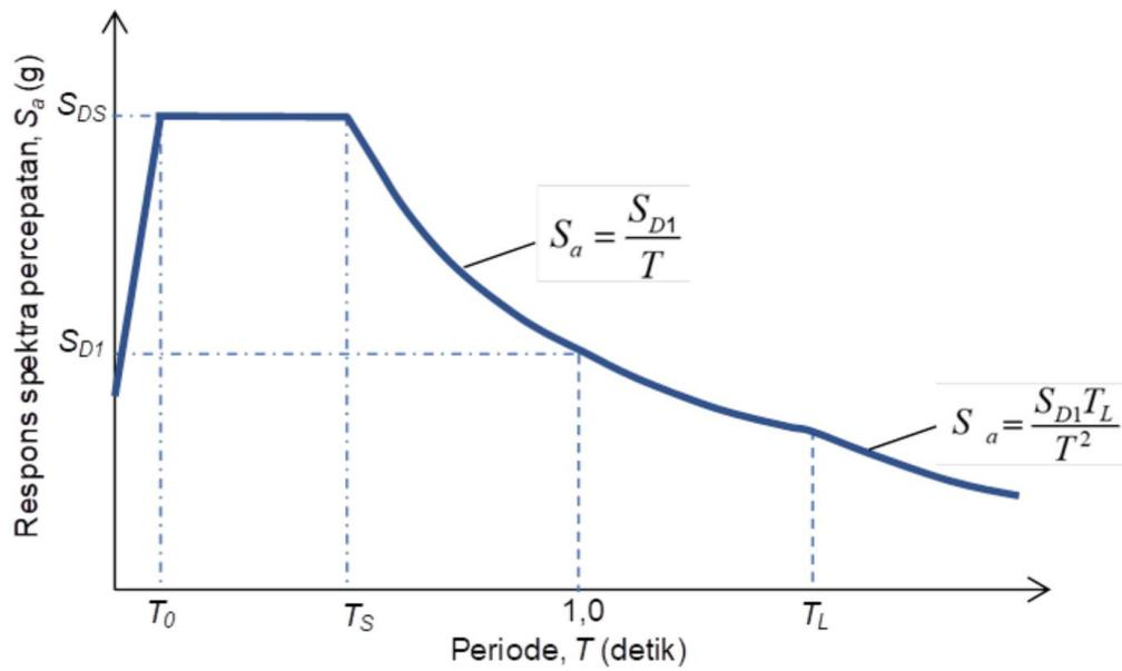
Figure 1. Design response spectrum
