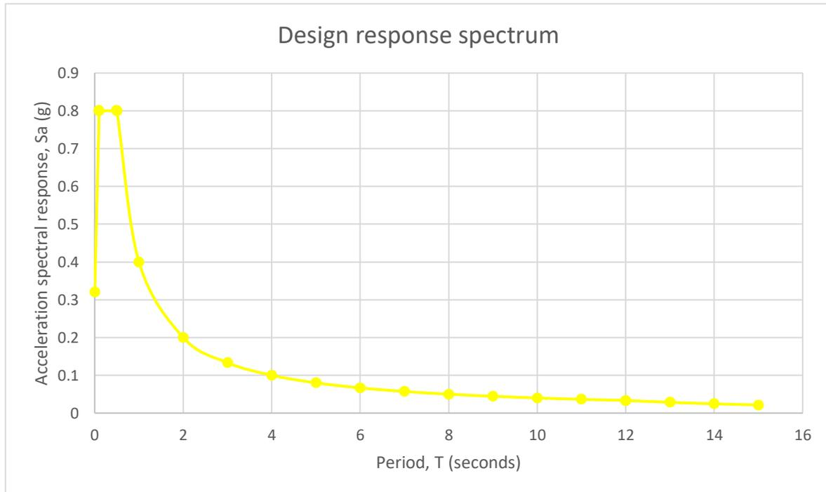
Figure 9. Design response spektrum for SE (soft soil)
