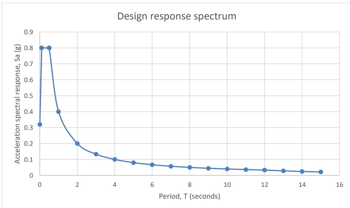
Figure 8. Design response spektrum for SD (medium soil)
