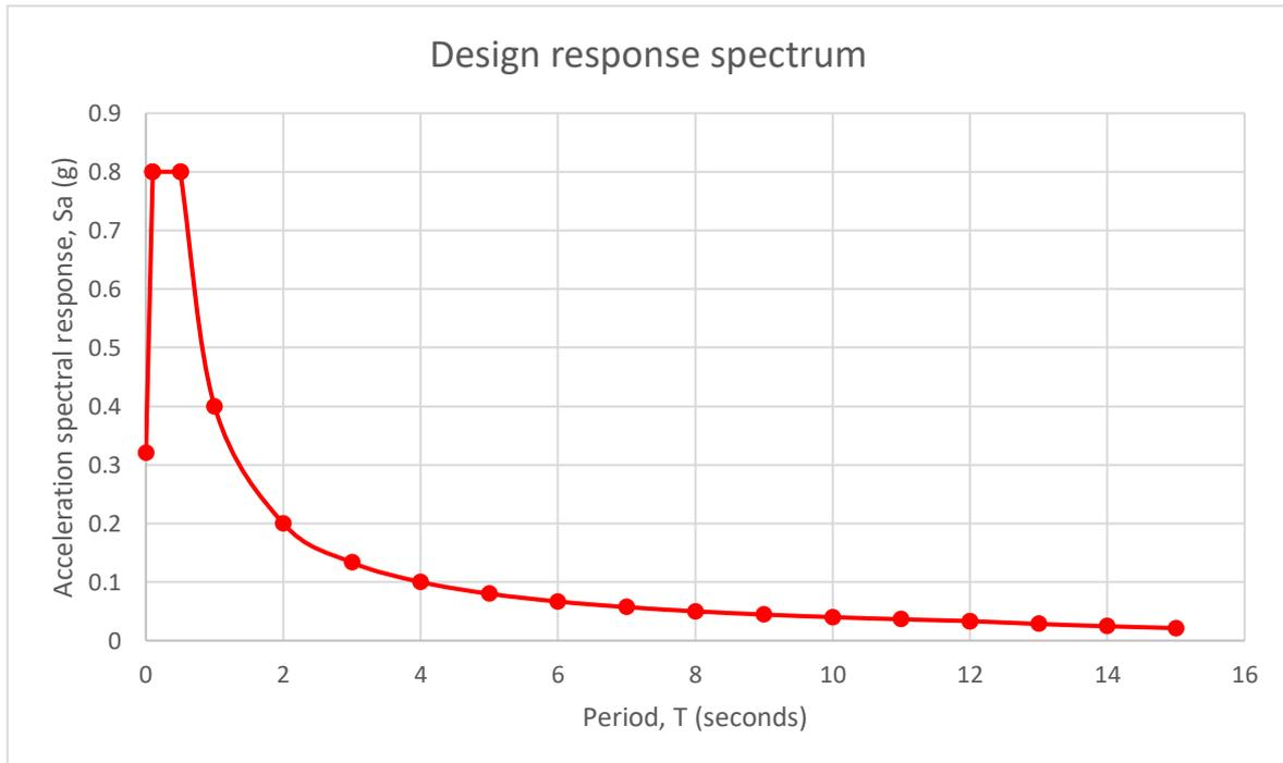
Figure 7. Design response spektrum for SC (hard soil, very solid and soft rock)
